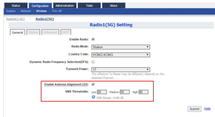
Figure 15 - LED indication for aligning the antenna
